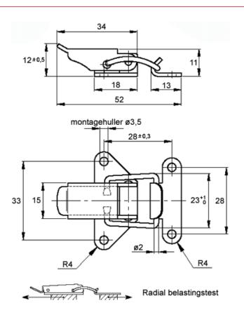
$\begin{array}{l} \text{Max load (N)} &= 550 \\ \text{Ultimate strength (N)} &= 1200 \end{array}$
